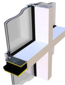
Siderise MI6 Insert: Through frame – sound transmission treatment using shaped composite high mass layer and acoustic foam inserts.
